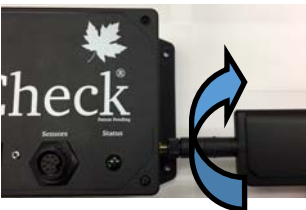
Figure 1a. Screw the antenna into the antenna port on the side of the SapCheck Controller.
