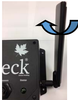
Figure 1b. Flip the antenna up. Optionally, rotate the antenna so that the flat side faces forward.
