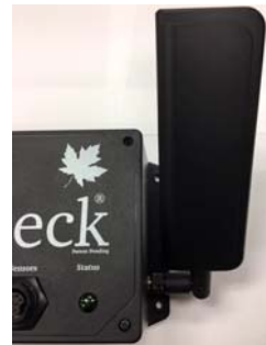
Figure 1c. Antenna installed in optional rotated orientation.
