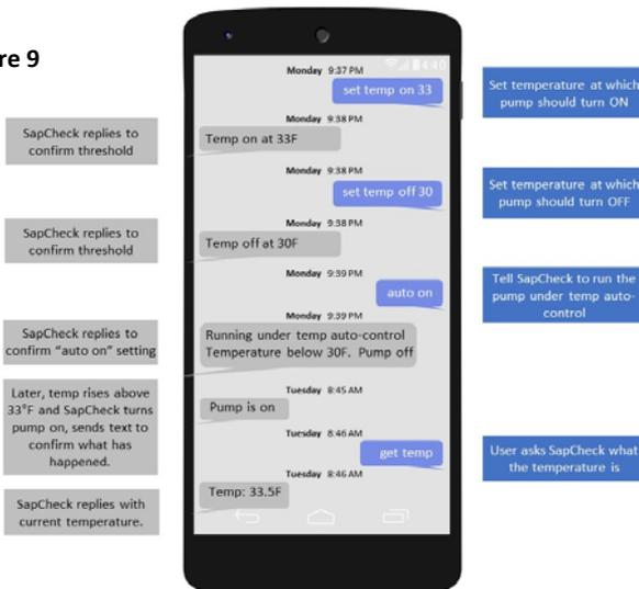
**REMOTELY STARTING / STOPPING VACUUM PUMP**
