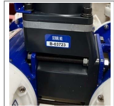
Pump serial number on side of motor Figure 1
