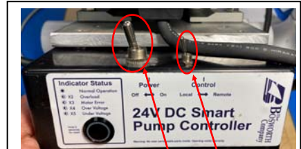
24 vdc Guzzler: On/off switch on left; remote control switch (smaller) on right.
