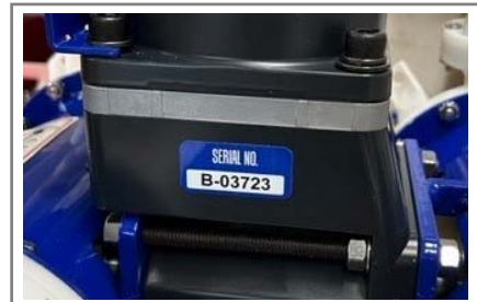
Pump serial number on side of motor
