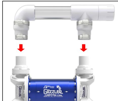
Attach the outlet manifold to the pump.
