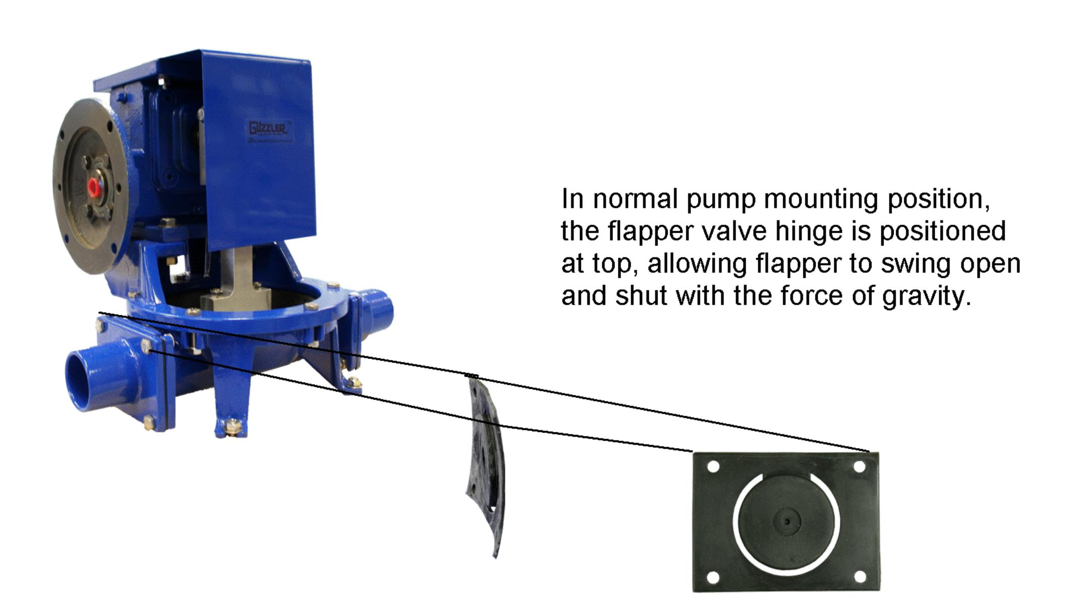
If pump is mounted upside down, remove inlet and outlet flanges and rotate flapper valves 180 degrees so that, in the pump's upside down orientation, the flapper valve hinge is still positioned at the top.
