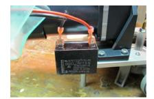
Figure 21. Connect wires to capacitor.
