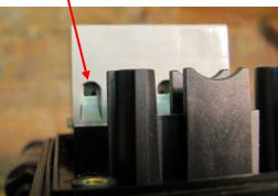
Figure 8. Open terminal block.
