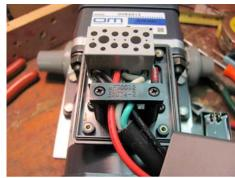
Figure 17. Reinstall strain relief strap over all 5 wires.
