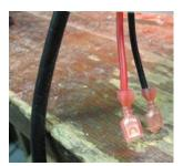
Figure 20. Crimp spade connectors onto wires.
