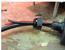
Figure 12. Thread the two 12" black and red cords through wire nut.
