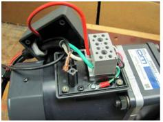
Figure 14. Connect green wire to  $\frac{1}{2}$  and the white wire to U1.
