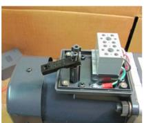
Figure 6. Remove strain relief strap.
